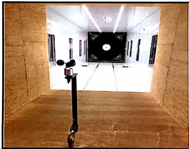
Photo of the wind tunnel setup. The cross-sectional area is 2.5m x 2.5m.
